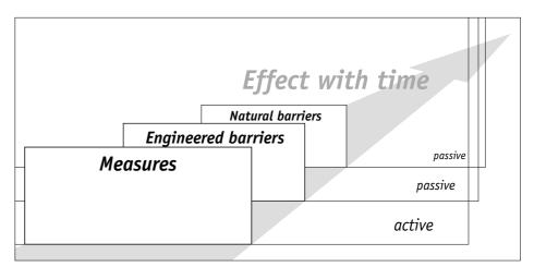
Figure 7: The safety systems for disposal of radioactive waste
