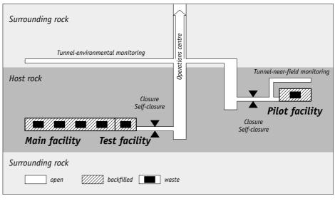
Figure 9: Schematic concept of the monitored long-term geological disposal facility: system elements
