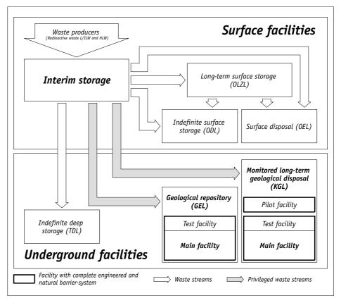
Figure 6: Disposal facilities at the earth's surface (surface facilities) and underground (deep facilities)
