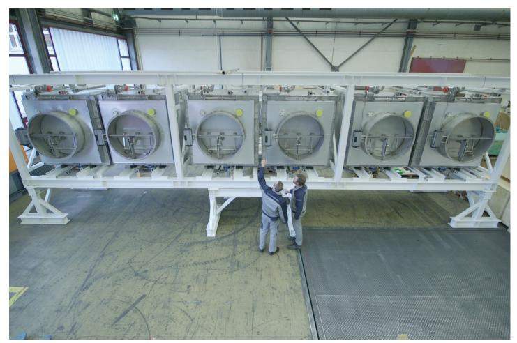
Six modules for  $CO_2$  capture are housed in a 40-foot shipcontainer. They are located at Climeworks company headquarters in Zurich-Oerlikon, ready to be installed at the pilot and demonstration facility in Hinwil in the Zurich Oberland region. The facility for  $CO_2$  capture shall go in operation in spring 2017. Photo: Climeworks
