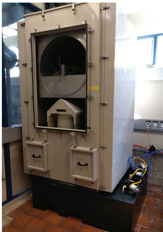
Functional model of the ZHAW absorption dryer: The system has a drying area of one square meter. Nettles, apple mint, peppermint and other herbs up to a moisture content of 12% can be dried in it. Photo: ZHAW
