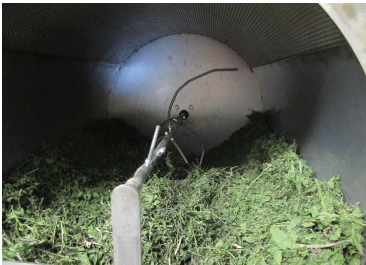
The agitator of the new drying system ensures that the herbs are dried evenly and that no pockets of moisture remain. Photo: ZHAW
