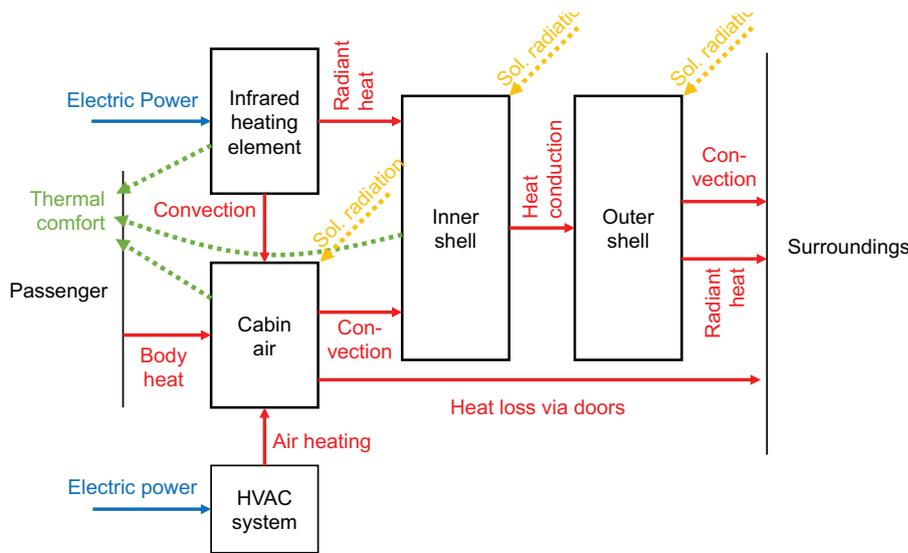
Illustration of the simulated heat flows in a public transport vehicle according to the model developed by Fabio Widmer at ETH. Illustration: Final report ISOTHERM
