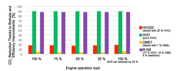
Fuels such as HVO and R100, which are virtually entirely of biogenic origin, can produce around 90% fewer  $CO_2$  emissions than diesel, depending on their origin. In HVO20 and OME7 fuel blends,  $CO_2$  emissions are reduced similarly depending on the proportion of biofuel they contain. Graphic: Final report ReVerDi/edited B. Vogel
