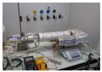
Empa researched the aspect of exhaust gas aftertreatment in the Re-VerDi project. In the picture: Test set-up to investigate the regeneration of the diesel particulate filter. Photo: Empa
