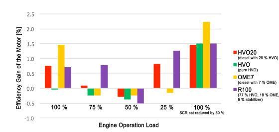
Since biofuels are less prone to form soot, they place less strain on the soot particle filter. The energy saved in this way can be converted into efficiency gains of the drive energy. Depending on the fuel or fuel mixture, this amounts to a good two percent. Graphic: Final report Re-VerDi/edited B. Vogel
