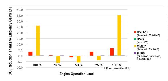
For the pure biofuels (HVO, R100), the additional CO<sub>2</sub> savings are hardly significant due to the efficiency gain. The situation is different for fuel blends containing only a proportion of biofuels (HVO20, OME7). Graphic: Final report ReVerDi/ edited B. Vogel
