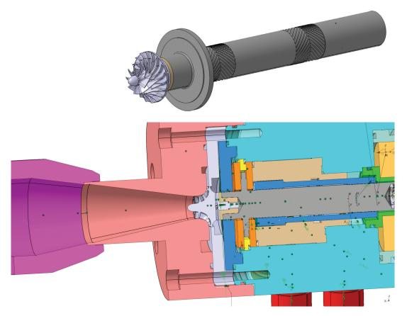
CAD representation of the rotor of a radial compressor: The bladed impeller is at the front , which radially deflects the heat pump's gaseous working fluid (flowing in from the left). The rotor is outfitted with V-shaped grooves, which create a gas film through the rotational movement, so that the rotor «floats» without touching the moving parts. Illustration: LAMD
