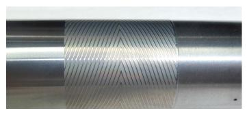
The V-shaped grooves are lasered or etched into the steel rotor. The pattern of the grooves has been chosen so that the air gap between the rotor and bearing is as large as possible, due to operational advantages. Illustration: LAMD
