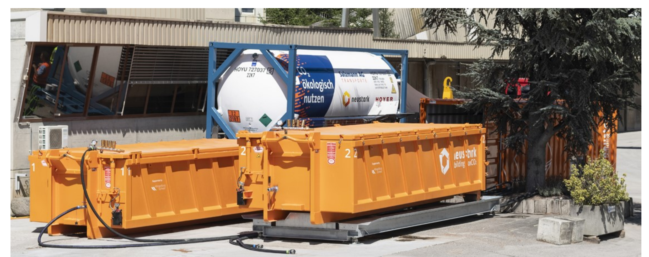
Fig 3: Pilot plant, operated at the Kästli concrete plant. It has been shown, that 1) 120-200t of concrete aggregate can be carbonated per day storing 2) 1000-1500 kg CO 2 . Furthermore, the material was used for the concrete material tests, as shown in Fig. 2.
