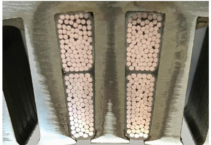
Modern shaped strand coil winding for the stator of an electric motor, designed as a plug-in winding. The winding is extremely compact and thus achieves a high fill factor of 56%. Photo: BRUSA
