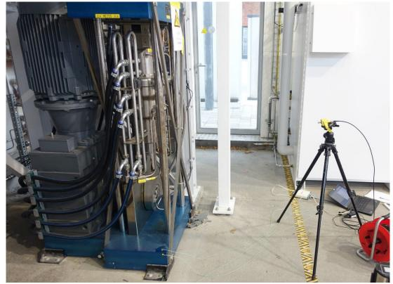
The compression of hydrogen to 700 bar produces noise that can affect the neighborhood. This noise can be shielded through a suitable sound insulation device. In the picture right: a device for sound measurement. Photo: Prose
