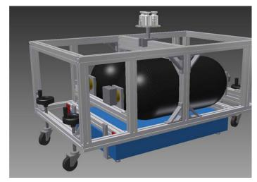
The mobile calibration device for hydrogen dispensers, as developed by the Swiss Federal Institute of Metrology in Wabern near Bern. The two tanks (black) are 91 cm long and have a diameter of 32 cm. In blue: the scale that can be used to precisely determine the weight of hydrogen in the two tanks. Illustration: Metas
