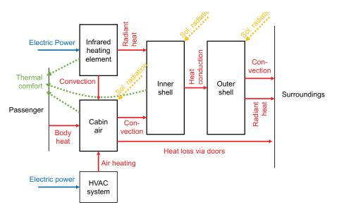
Illustration of the simulated heat flows in a public transport vehicle according to the model developed by Fabio Widmer at ETH. Illustration: Final report ISOTHERM
