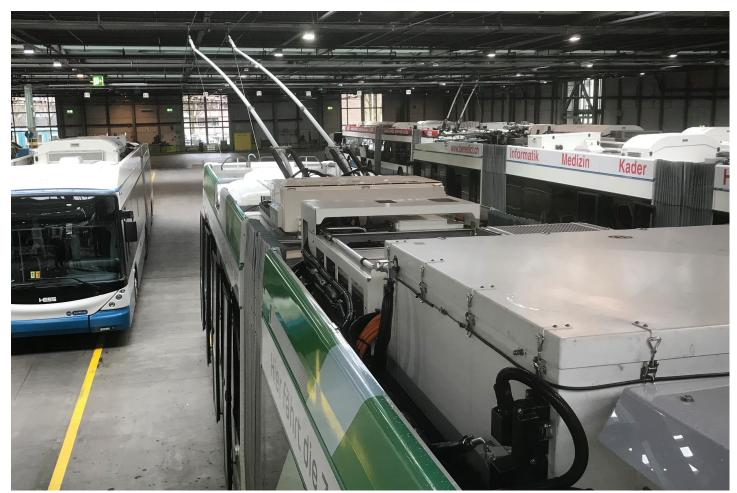
The battery on the roof enables this trolleybus to travel routes without overhead power lines. Photo: B. Vogel
