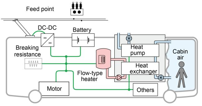
Energy system of a trolleybus that, thanks to a battery, can also travel to areas without an overhead power line. An ETH study investigated, among other things, how the service life of the battery can be extended by clever charge/discharge management or by optimized operation of the heating system. Green stands for electrical connections, red for hot water, blue for air. Illustration: ISOTHERM final report
