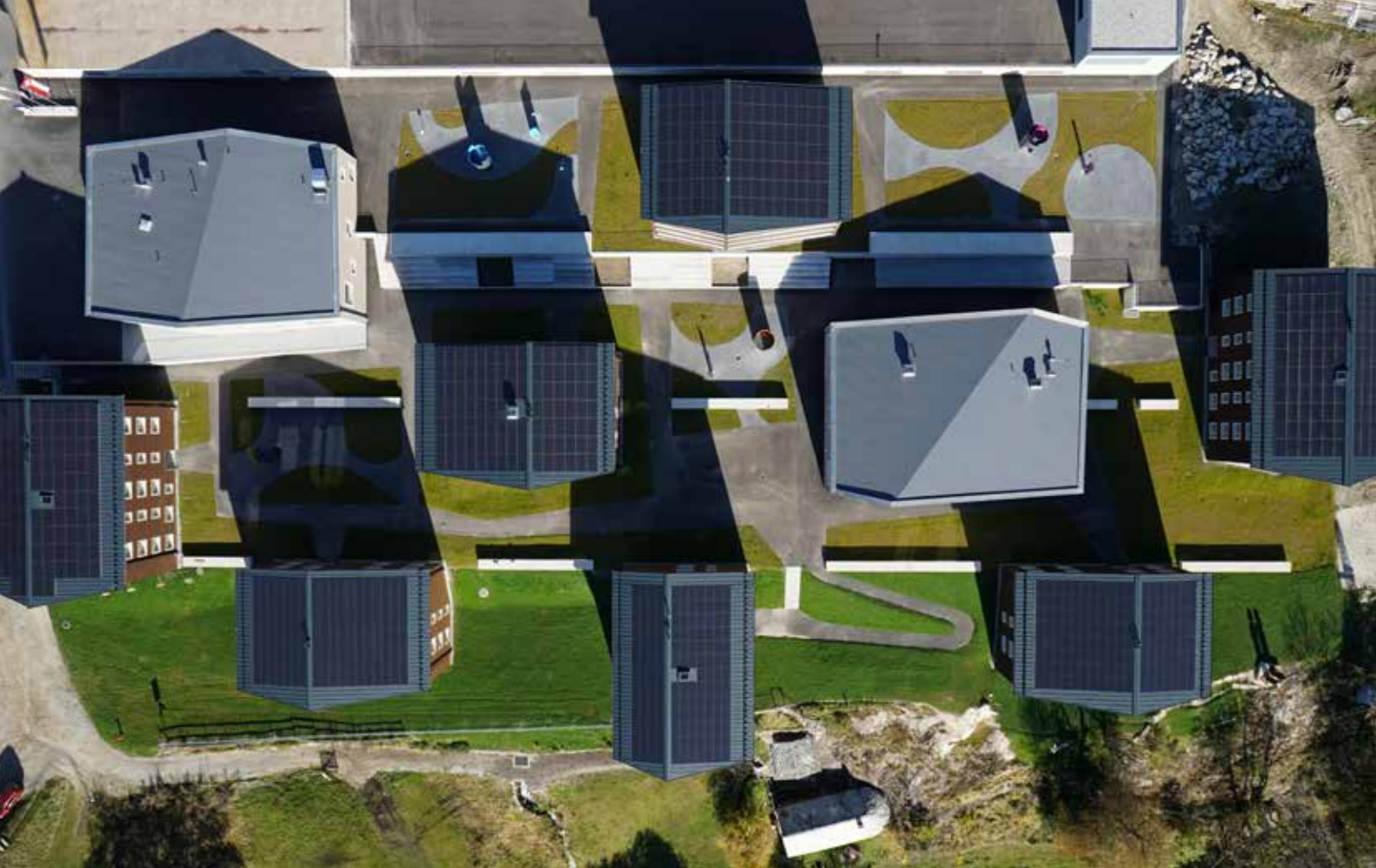
Reka Holiday village of Blatten (VS): The roofs are oriented to the east and west so that the solar energy yield is at its highest in the morning and afternoon, i.e. when energy demand in the holiday village is at its daily peak.
