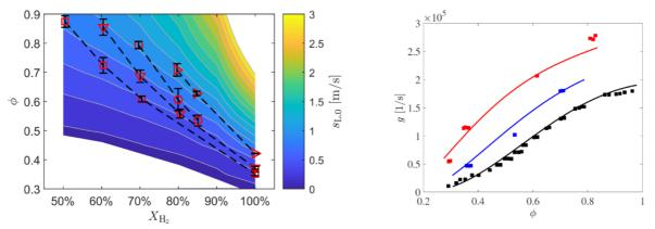
Figure 1: On the left, the flashback limits at p=2.5 bar and Tpre=200 °C [1]. On the right, experimentally measured boundary layer flashback limit data of Eichler [2] (squares) compared to the model developed in this work (lines). The flashback limits cover three discrete preheat temperatures of 20 °C (black), 200 °C (blue), and 400 °C (red).
