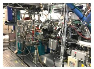
6-cylinder Diesel-Engine on a test rig with DME injection and EGR blower Hardy, FPT; Soltic, Empa
