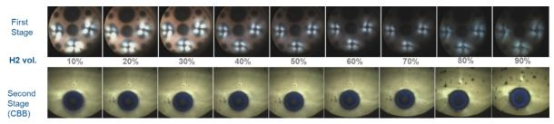
Operation concept for highly reactive fuels (hydrogen): the first stage flame temperature is tuned for optimum boundary conditions of the second stage (Center Body Burner), maintaining maximum combustor exit temperature for best engine performance at low NOx emissions. Images from full-scale high-pressure testing.
