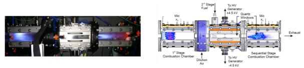
Figure 1: Atmospheric pressure sequential combustor.
