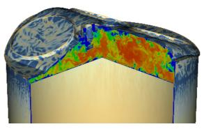
DNS of full scale pent-roof engine: temperature distribution on cut planes, wall heat flux on surfaces Giannakopoulos, Frouzakis, Keskinen, Bolla, Wright and Boulouchos, LAV ETHZ
