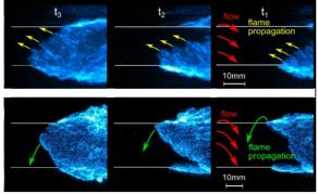
Two distinct flame propagation pathways in a gas turbine burner: (a) 50° (b) 65° Swirler Ebi, Energy System Integration, PSI
