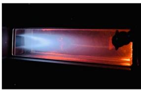
Combustion of Hydrogen in the hot vitiated flow of a laboratory sequential combustor Solana Pérez, Shcherbanev, Noiray, CAPS ETHZ
