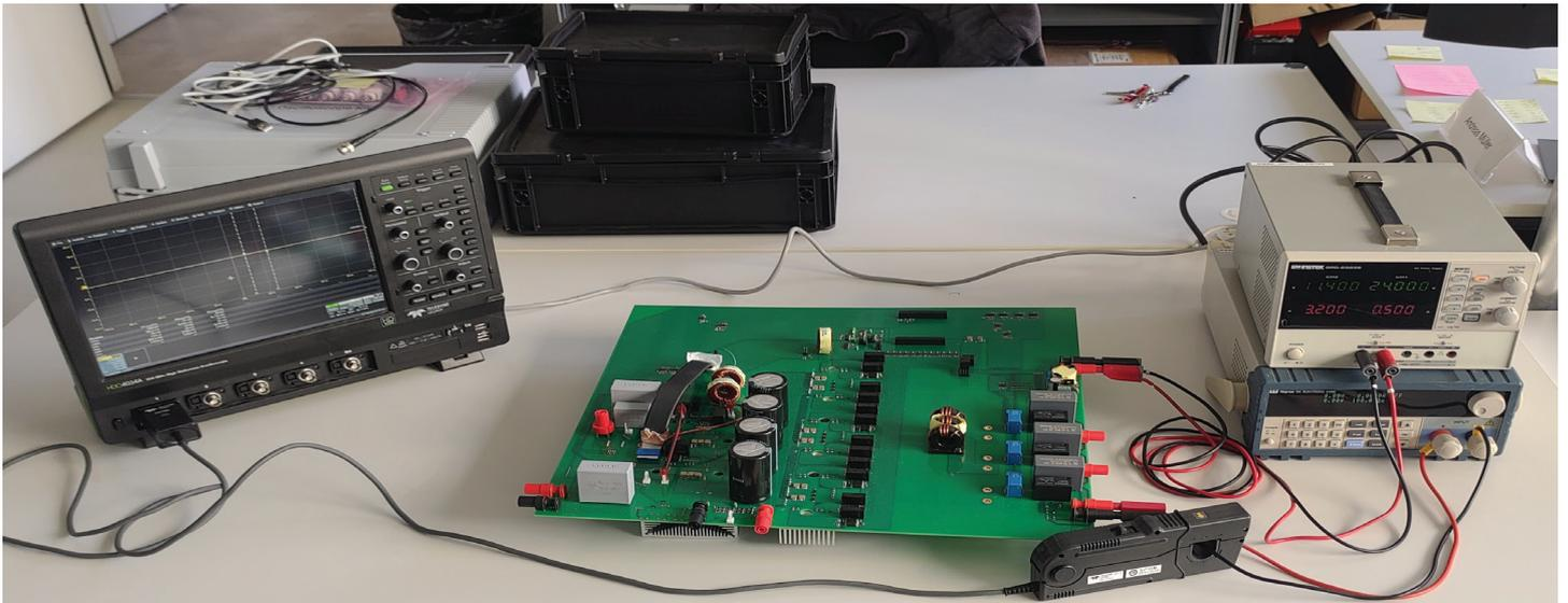
Test setup of the ZHAW research group led by Prof. Andreas Heinzlmann for measuring the efficiency of DC/DC converters with new wide-bandgap semiconductors in solar inverters for single-family home systems. Photo: ZHAW IEFÉ
