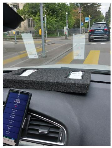
The device on the left under the windshield measures high-frequency electromagnetic fields, while the device on the right measures low-frequency magnetic fields. Photo: Fields at Work
