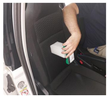
Measuring device for low-frequency magnetic fields on the back seat. Since the strength of EMF fields varies by location, three positions were measured: directly on the backrest, about 5 cm from the backrest, about 10 cm from the backrest (shown). Photo: Fields at Work
