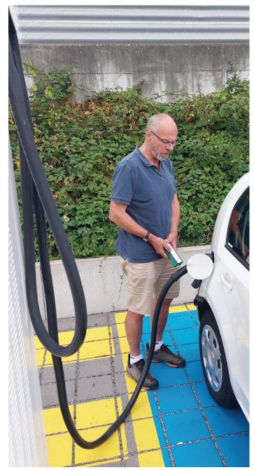
Measurement of magnetic fields during charging. Photo: Fields at Work
