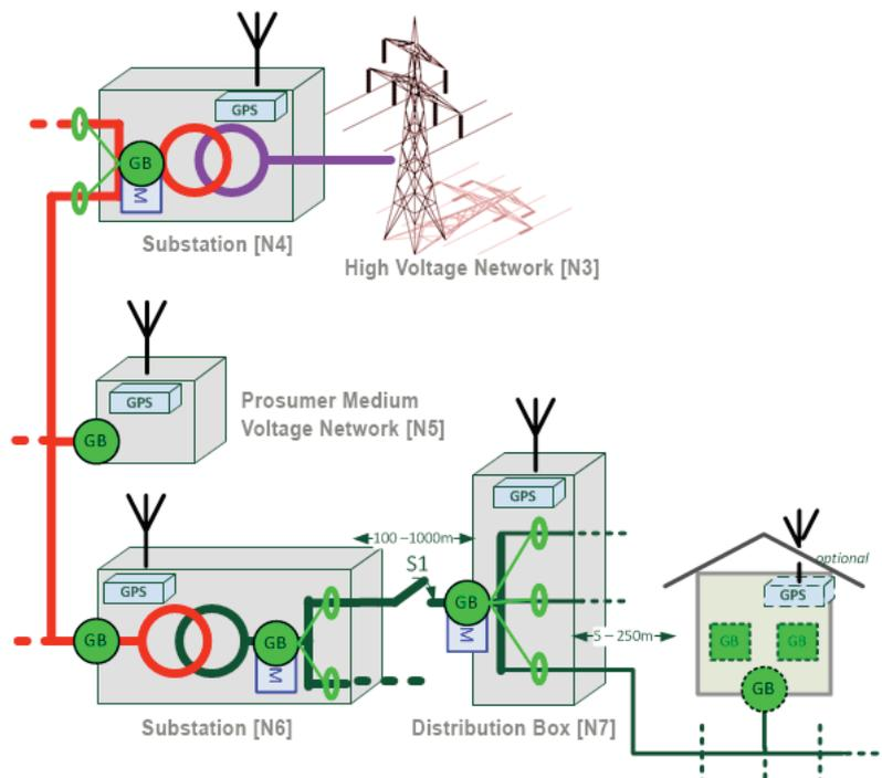
*Gridboxes are installed at various points in the medium and low voltage grid, enabling system monitoring and also control of flexible loads and generators. Photo: SCS*
