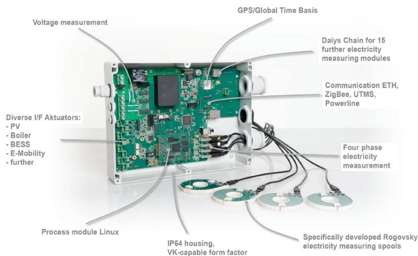
*The Gridbox base module and four Rogowski coils for contact-less electricity measurement (front right). Photo: SCS*
