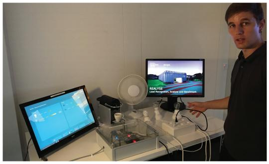
*iHomeLab* Project Leader Lukas Kaufmann with the demonstrator NIALM system: There are two devices turned on (right screen and fan); on the screen on the left is displayed the class to which the two devices belong, also the current power consumption. Photo: B. Vogel
