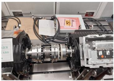
The Roadrunner project, in which bus manufacturer Hess and the ABB Group are developing a converter based on WBG semiconductors, was launched in 2019. The photo on the left shows a prototype of the converter. The picture on the right shows the test bench on which, among other things, journeys can be simulated. Photos: ABB Schweiz AG
