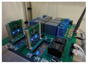
The team of Prof. Dr. Nicola Schulz has built and tested a DC-DC converter (22 kW; DC voltage 700 V to DC voltage 400 V) based on SiC at the University of Applied Sciences Northwestern Switzerland (Windisch site) in a project supported by the SFOE. Photo: FHNW
