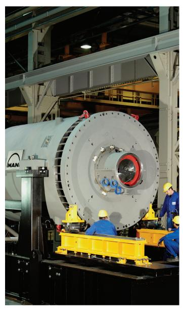
Example of a radial compressor, as they could be used in an compressed air storage plant. Such compressors are widely used in the oil/gas business, in steel production or in the separation of air into nitrogen and oxygen. Source: MAN Energy Solutions Schweiz AG
