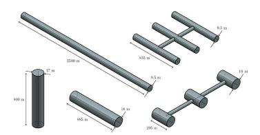
A commercial compressed air storage plant with a capacity of 500 MWh would require a rock cavern with a volume of 177,000 m<sup>3</sup>, which corresponds to a sphere with a diameter of 70 m. Apart from a sphere, other shapes are also conceivable, as shown in the diagram. Which shape is most suitable is being investigated in a SFOE project that is currently still ongoing. Illustration: Philipp Roos / Andreas Haselbacher
