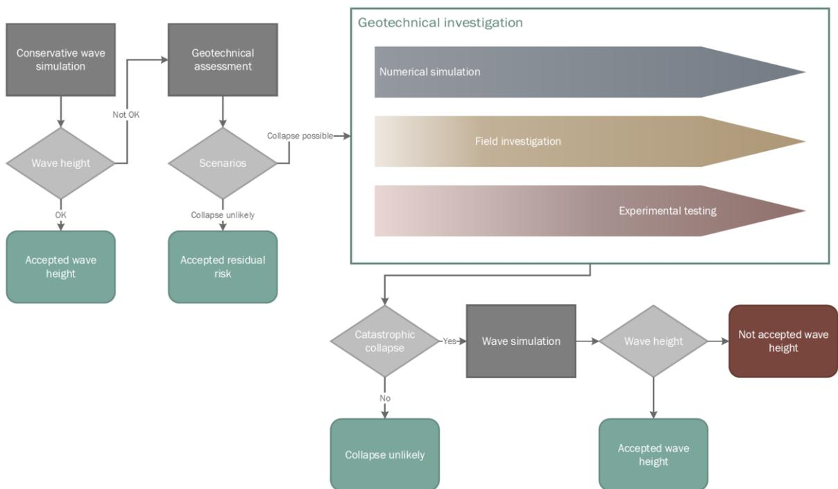
Figure 5.1: General procedure for the assessment of a catastrophic collapse
