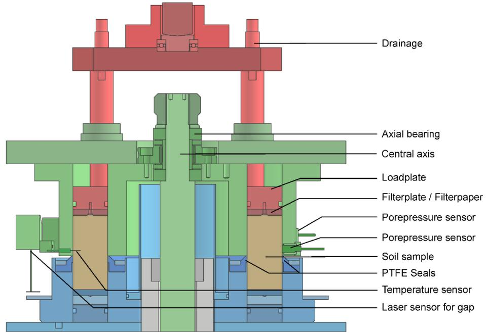
Figure 3.6: Cross section of the ring shear box showing all the main parts and sensors.
