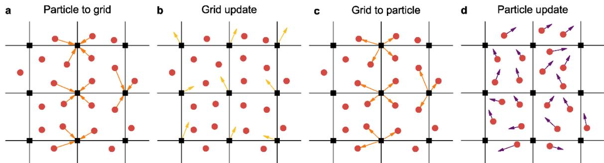
**Figure 3.2:** General 4-step algorithm of the MPM: (a) transfer of mass, linear momentum and forces from the material points to the grid, (b) solving the equation of motion on the grid, (c) transfer the updated grid velocities back to the material points and (d) evolve the material points and updated the deformation and stress state (after Soga et al., 2016).
