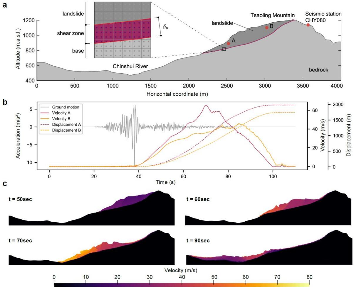
**Figure 3.11:** Simulation of the catastrophic Tsaoling landslide. Cross section of the landslide model including the selected output points (after Tang et al. (2009)) (a). Evolution of velocities and displacements of two selected points in the landslide (b). Displacements and velocity distribution at selected times during the landslide failure (c).
