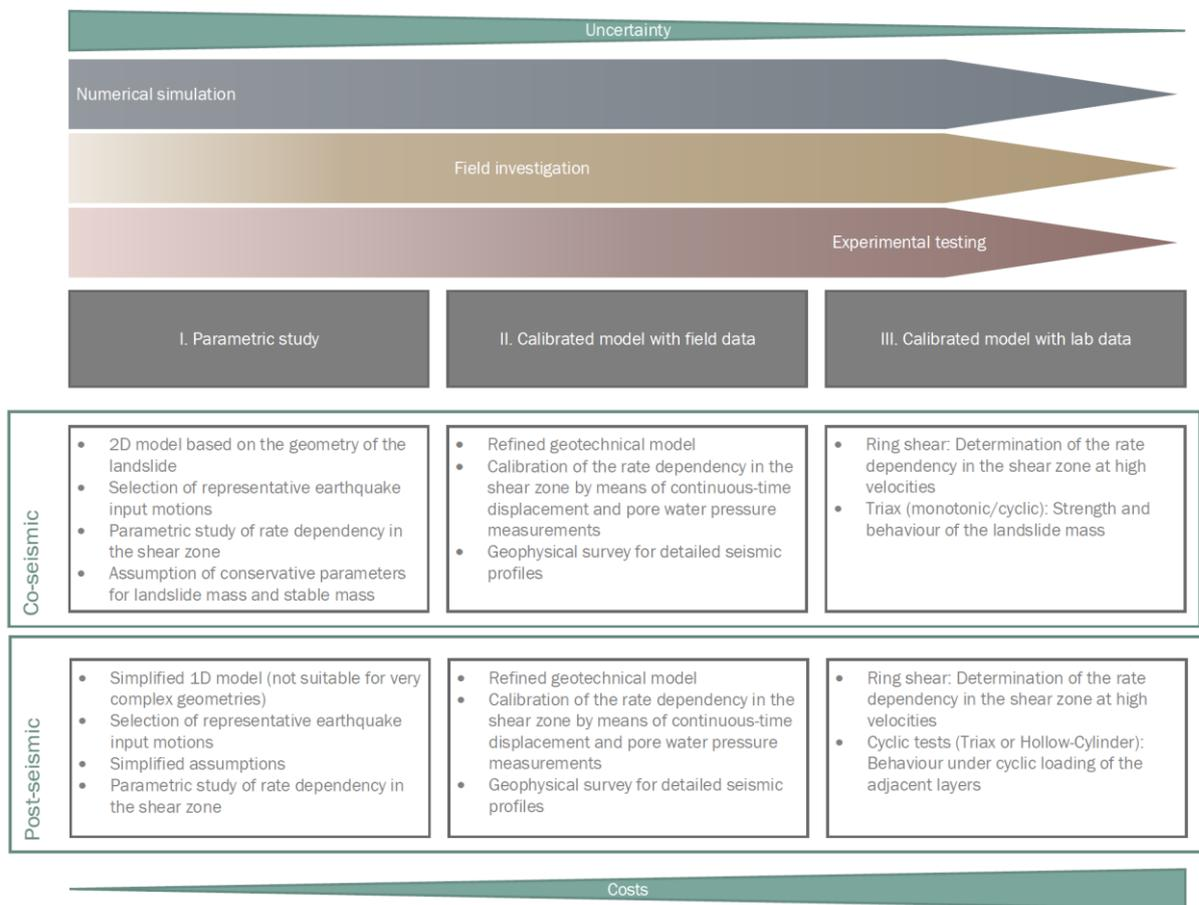
Figure 5.3: Procedure for the assessment of co- and post-seismic displacements
