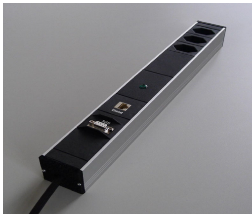
Figure 2: Prototype of an intelligent switching panel for server management (source: EMT AG, Ermatingen)
