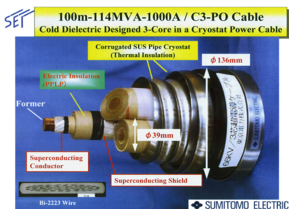
Figure 1: Prototype HTSC cable from Sumitomo (source: Sumitomo Electric, Japan)
