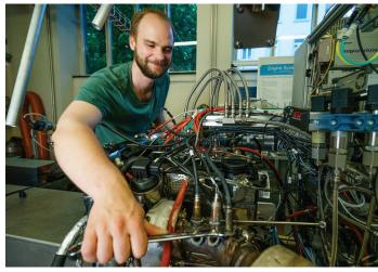
As part of his doctoral thesis at ETH Zurich, Richard Hutter carried out experiments on a modified diesel engine (dual fuel engine): In the engine, self-igniting diesel is used to ignite difficult to ignite methane. Photo: IDSC
