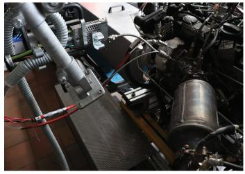
Close-up of the NextICE engine test bench at ETH Zurich: The cables lead to a measuring probe with which unburned methane is measured. The pollutants are removed in the three-way catalytic converter on the right. Photo: B. Vogel
