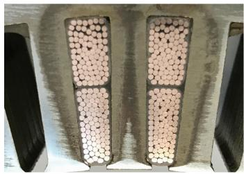
Modern shaped strand coil winding for the stator of an electric motor, designed as a plug-in winding. The winding is extremely compact and thus achieves a high fill factor of 56%. Photo: BRUSA
