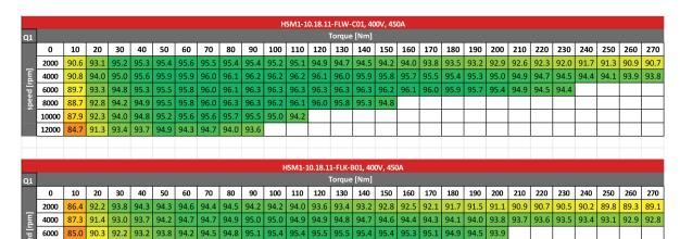
Efficiency as a function of revolution speed and load point for the electric motor with plugin winding (latest version/top or earlier version/middle) and the electric motor with pull-in winding (bottom). The table shows that the new motor achieves very good values of 96 and more percent in the partial load range of a vehicle weighing 3.5 to 7.5 t (70-120 Nm at 4000-8000 rpm).
