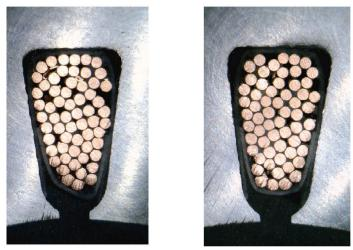
Earlier generation of a shaped strand coil-winding installed in the stator of an electric motor (photos: two different grooves of the same stator in cross-section). The winding is realized as a pull in winding and achieves a fill factor of approx. 40%. Photo: BRUSA
