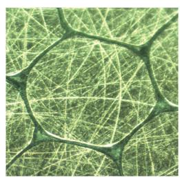
The microscopic image shows the cross-section of a single strand of a stator winding: The strand takes on a hexagonal shape because of mechanical shaping. Photo: BRUSA
