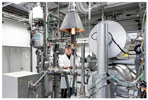
In this laboratory, PSI researchers produce energy-rich gas from wood, a natural raw material. The process converts wood into synthetic natural gas, which is fed into public gas pipelines. The energy is thus made available for power generation in gas power plants or car engines. At the same time, wood is a very environmentally friendly energy source, as the gasification process is carbon-neutral. (Scanderbeg Sauer Photography)
