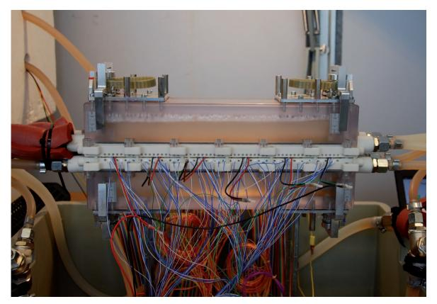
Waste heat from waste water can be converted into electricity by thermoelectric generators. Waste heat is created in many processes in business and industry, including in energy conversion. At the ETH Zurich, a one-kW demonstrator is used to assess basic feasibility and evaluate efficiency. By applying this process in concrete situations, scientists want to demonstrate that is is possible to use waste heat from data centres and heat from geothermal sources.
