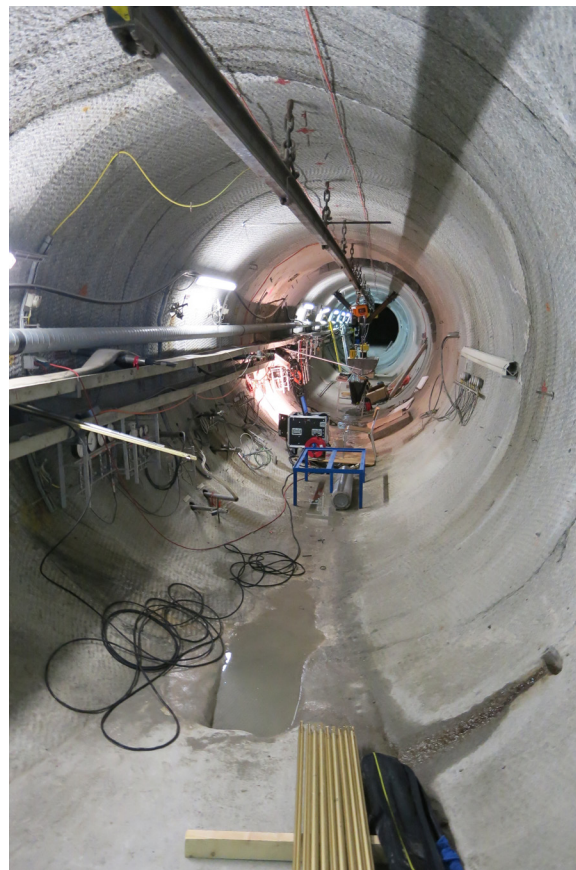
Application-oriented geological research is being carried out at the Grimsel rock laboratory in the Bernese Highlands with the aim of exploring geothermal resources in Switzerland. Geophysical tests are being conducted in tunnels at the laboratory in order to comprehensively characterise the rock formations before a controlled test can be initiated to pave the way for hydraulic stimulation.
