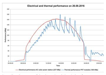
Recording the course of the thermal and electrical performance over a day. The fluctuations of the thermal power supplied by different supply temperatures, which are caused by the operation of the heat pump. Graphic: ZHAW Wädenswil
