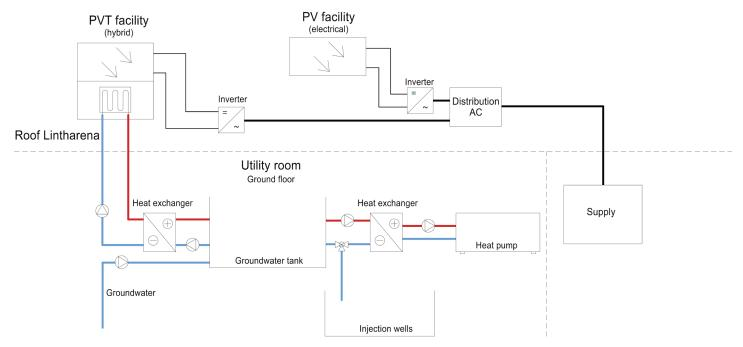
Functional diagram of the solar system on the roof of Lintharena sgu: The electricity from the PV panels (top center) is fed into the grid. The PVT collectors (top left) produce electricity and heat. The heat passes through a heat exchanger in the groundwater tank and is used from there to operate the heat pump. Subsequently, the groundwater in the soil is again supplied via the injection wells. Illustration: ZHAW Wädenswil
