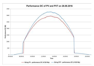
Comparison of DC power between a PV and a PVT cable with the same number of panels and thus the same electric nominal output shows that throughout the day, one fine day in August, the cooling of the PVT panels has a positive effect on performance. The PVT cable produced about 10% more electrical energy than the PV cable. Graphic: ZHAW Wädenswil
