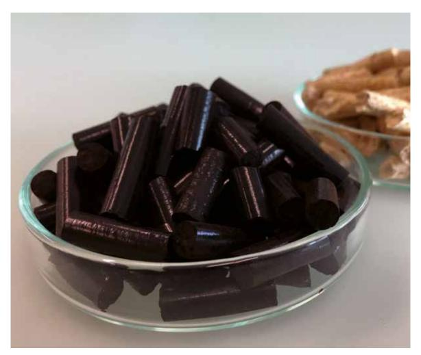
By means of hydrothermal carbonisation, organic residues can be converted in an ecologically, climate- and hygiene-friendly way to be used for energy generation or as plant nutrients for agriculture. The figure shows carbonisates from slurry in pellet form with an energy density of 10-12 GJ/m<sup>3</sup> (source: FHNW).
