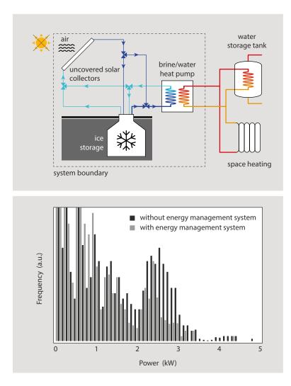
Test arrangement for a heat pump with heat supplied from a solar collector (uncovered tube absorber) in combination with an ice storage tank. The ice storage tank simultaneously serves as a heat storage tank for solar heat (graphic according to FHNW).
