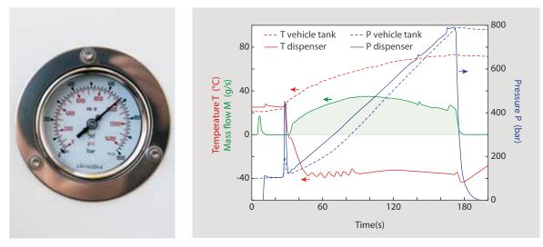
Since 2016, fuel cell vehicles can be refuelled in Switzerland with 700 bar hydrogen. In accordance with the SAE J2601 protocol, such a refueling takes only a few minutes. To prevent the temperature in the vehicle tank from rising too much, the hydrogen must be pre-cooled at the filling station. The mass flow during such a refuelling corresponds to a power flow of more than 5 MW (Source: Empa, graph based on Empa data).
