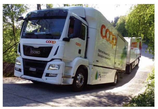
Prototype fuel cell truck developed by Esoro in cooperation with Swiss Hydrogen: Successful drive-off test at a slope of 30 % and a total weight (truck plus trailer) of 35 tons (source: Esoro).
