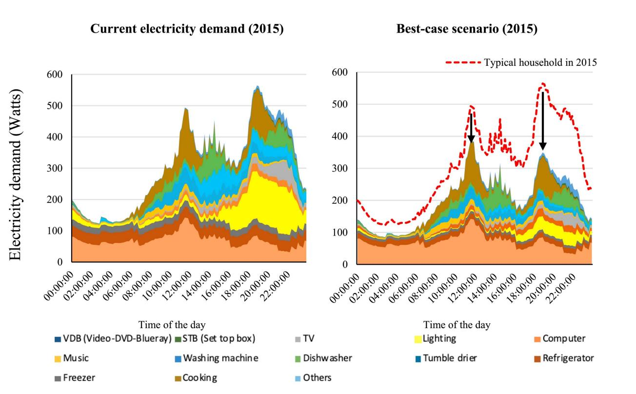
Comparison of domestic appliance electricity demand profiles for a mean Swiss household in 2015 with a best-case scenario in which all the appliances are replaced with the currently most efficient version.
