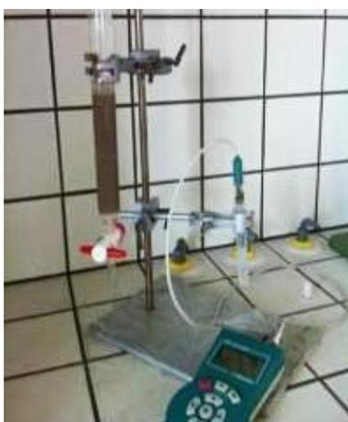
**Figure 2:** Photograph of the ion exchange process of sodium silicate to produce a silicic acid sol
