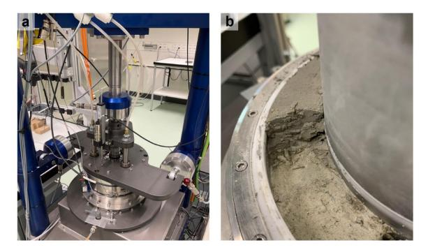
Figure 3.7: Photos of the ring shear apparatus (a) and the shear zone and PTFE seals (b).
