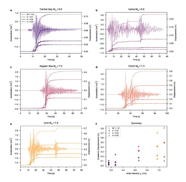
**Figure 3.9:** Results from parametric study. Ground acceleration and evolution of co-seismic displacements calculated at the bottom of the landslide for different earthquake events (a-e). The simulations are performed each for a rate independent shear zone and for three different rate dependency parameter A. Summary plot showing the final co-seismic displacements against the corresponding Arias intensity (f). Reprinted from Kohler et. al. (2023), where further information can be found.
