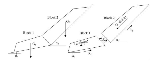
Figure 2.2: Simplified representation of landslide with varying inclination as two blocks.
