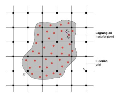
Figure 3.1: Lagrangian MPM discretization of a continuum and the Eulerian computational grid.
