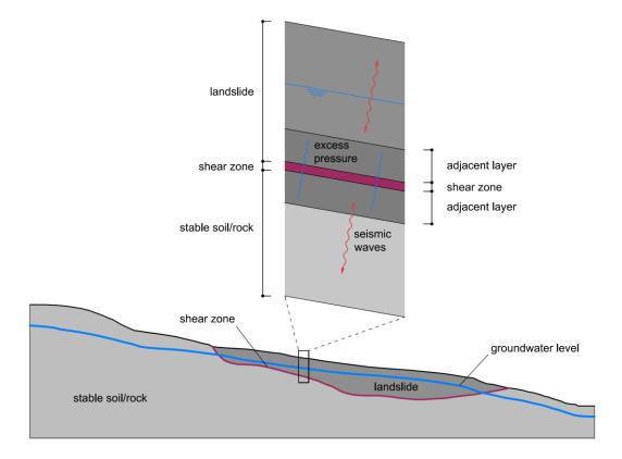
Figure 2.1: Schematic representation of a creeping landslide
