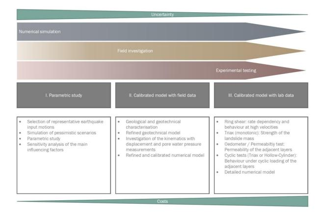
Figure 5.2: Detailed procedure for the geotechnical investigation.
