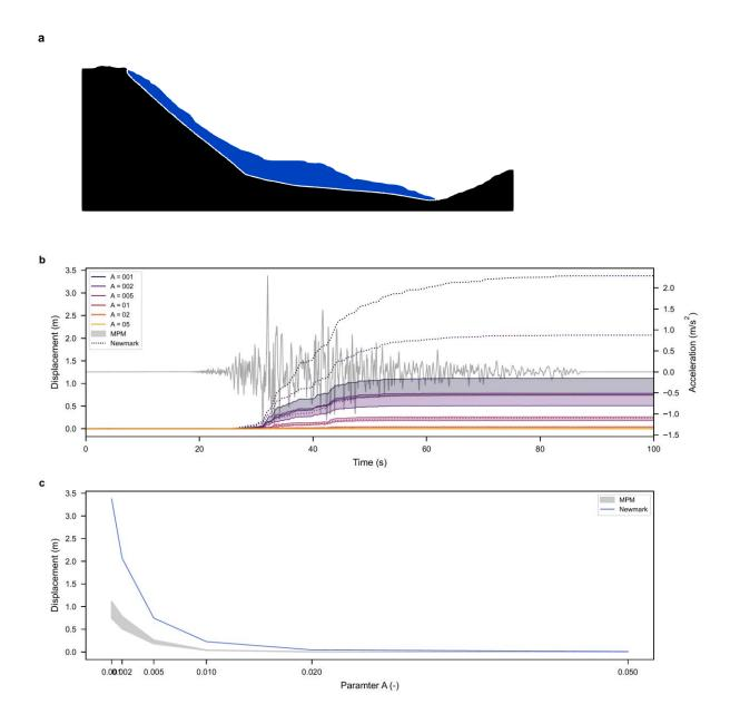
**Figure 5.6:** Co-seismic displacement for the Brienz landslide in Switzerland. (a) Geometry of the Brienz landslide. (b) and (c) comparison of the MPM simulation with a simplified Newmark for different rate dependency parameters A. The MPM simulation provides co-seismic displacements at each point of the landslide. The range of displacement is therefore represented as a hatch.
