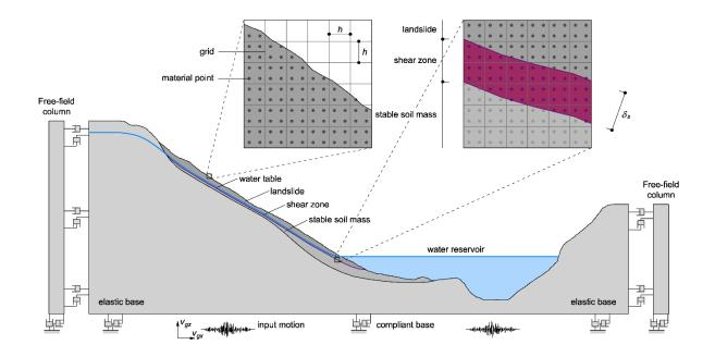
**Figure 3.3:** MPM landslide model. Schematic view of the MPM model of the landslide based on the Marsc landslide at the Luzzone reservoir, including the free-field columns at the lateral boundaries. The grid size is denoted with *h* and the thickness of the shear zone with  $\delta_s$ . The earthquake motion is applied by a vertical and horizontal component denoted with ground velocities  $v_{gx}$  and  $v_{gx}$ .
