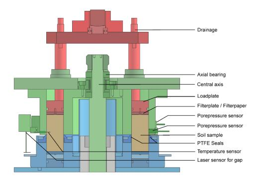
Figure 3.6: Cross section of the ring shear box showing all the main parts and sensors.
