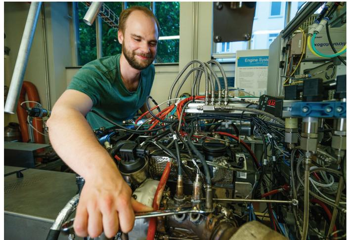
As part of his doctoral thesis at ETH Zurich, Richard Hutter carried out experiments on a modified diesel engine (dual fuel engine): In the engine, self-igniting diesel is used to ignite difficult to ignite methane. Photo: IDSC
