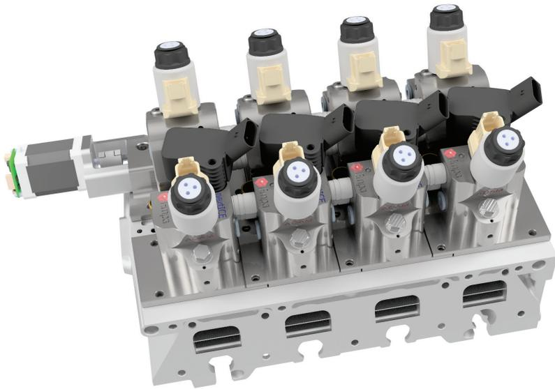
On the left: CAD design of the fully variable valve train.
