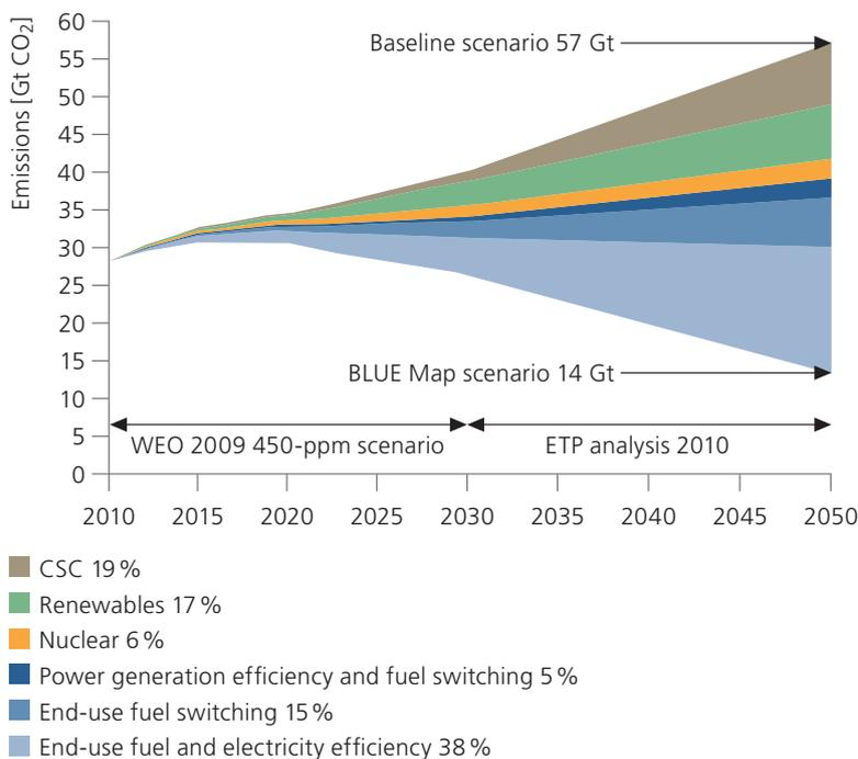
Diagram 1: Key technologies for reducing carbon emissions under the IEA BLUE Map scenario. (IEA Energy Technology Perspectives 2010)
