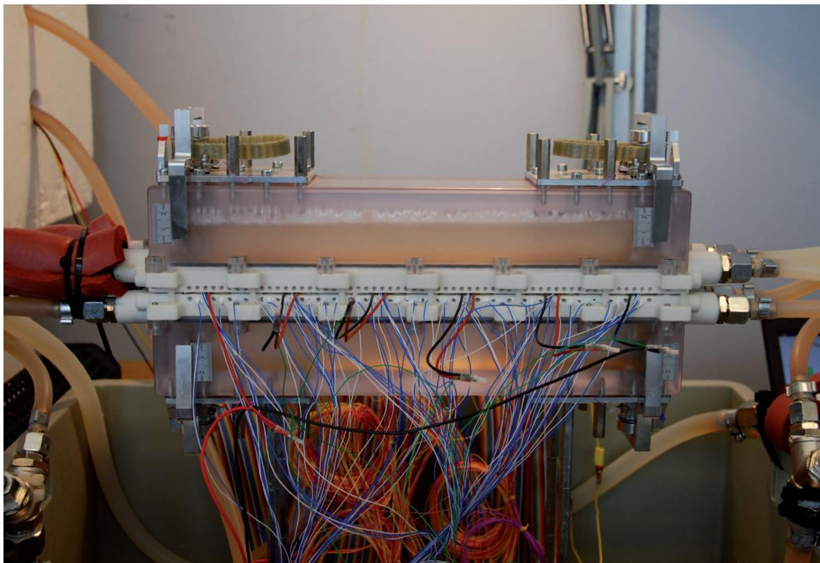
*Waste heat from waste water can be converted into electricity by thermoelectric generators. Waste heat is created in many processes in business and industry, including in energy conversion. At the ETH Zurich, a one-kW demonstrator is used to assess basic feasibility and evaluate efficiency. By applying this process in concrete situations, scientists want to demonstrate that it is possible to use waste heat from data centres and heat from geothermal sources.*
