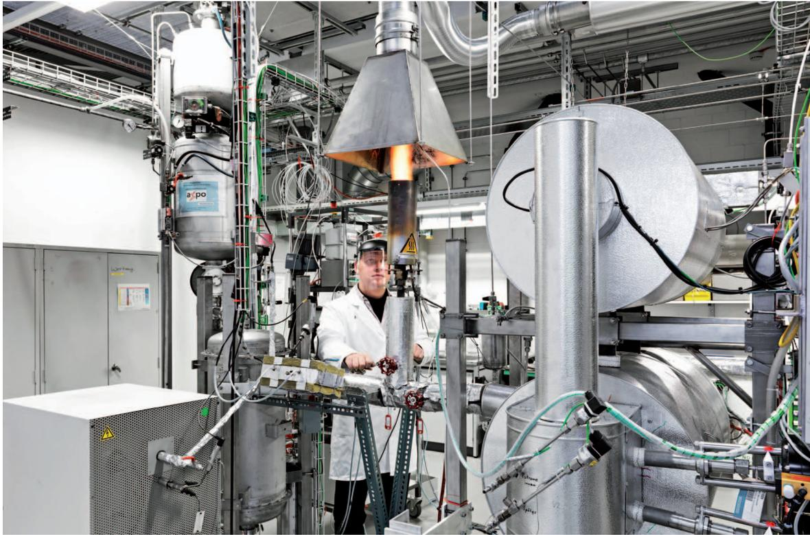
*In this laboratory, PSI researchers produce energy-rich gas from wood, a natural raw material. The process converts wood into synthetic natural gas, which is fed into public gas pipelines. The energy is thus made available for power generation in gas power plants or car engines. At the same time, wood is a very environmentally friendly energy source, as the gasification process is carbon-neutral.
