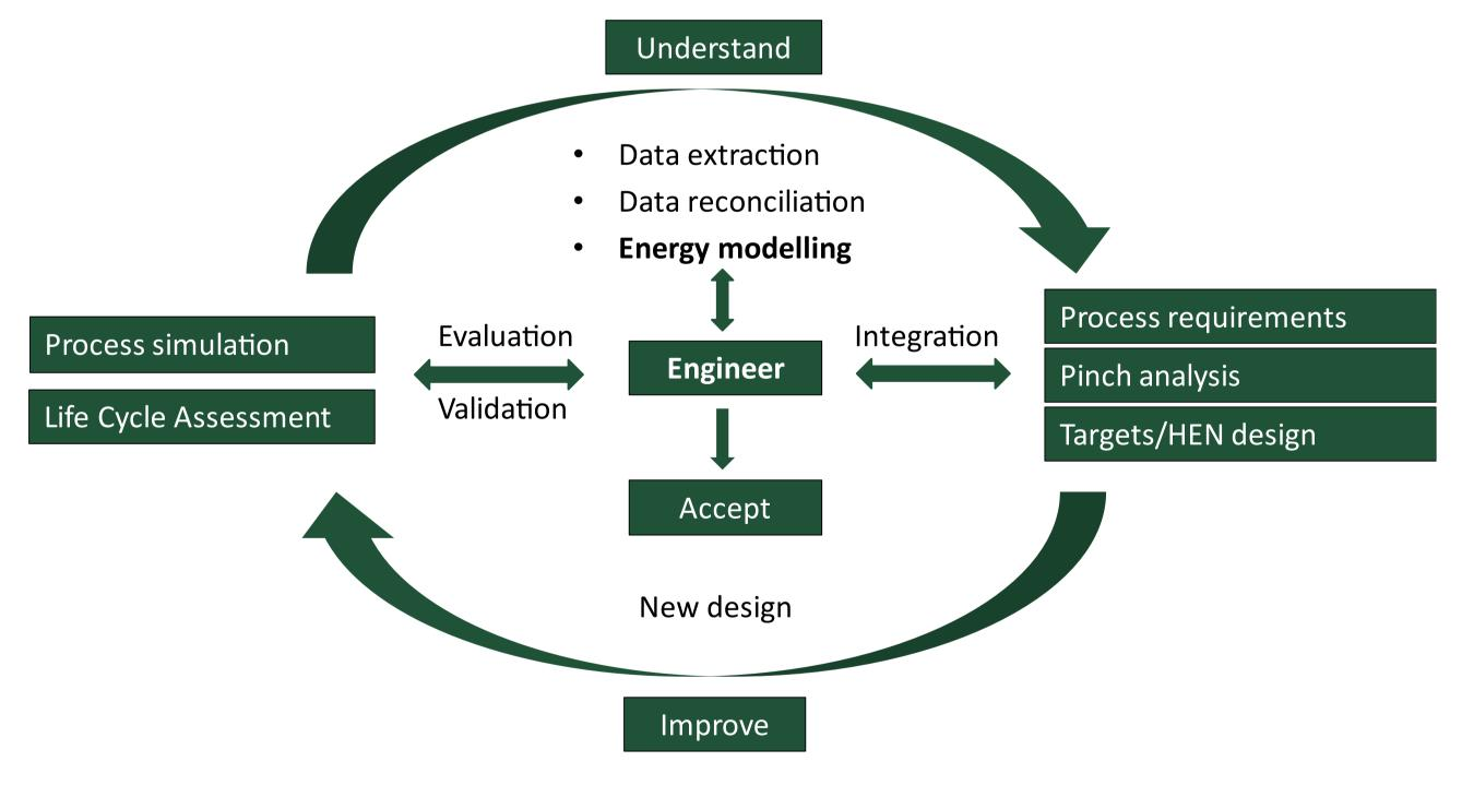
The novel iterative method incorporates and extends **process** simulation tools, PA, costs optimization and **ecological** considerations (life cycle assessment LCA), and heat exchanger network (HEN) design. The key to this workflow is keeping the engineer central.
