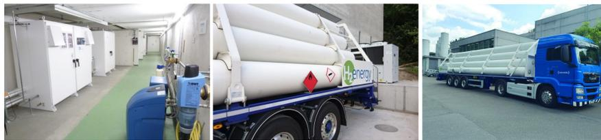
Production (left), compression (middle) and transport (right) of H<sub>2</sub> for the supply of the fueling station at Hunzenschwil
