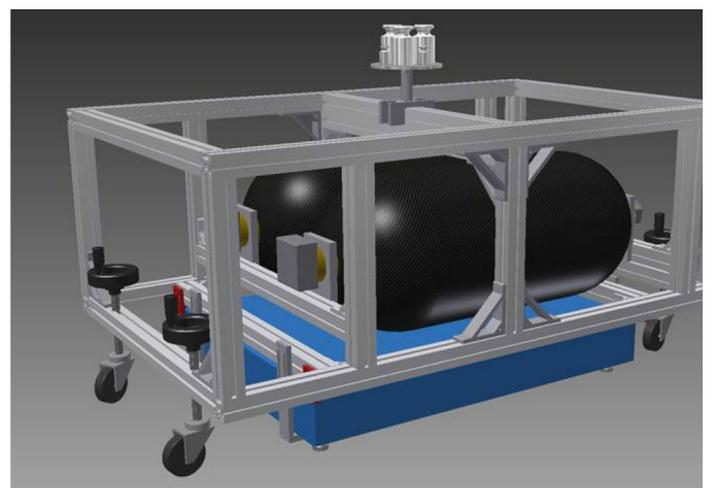
The mobile calibration device for hydrogen dispensers, as developed by the Swiss Federal Institute of Metrology in Wabern near Bern. The two tanks (black) are 91 cm long and have a diameter of 32 cm. In blue: the scale that can be used to precisely determine the weight of hydrogen in the two tanks. Illustration: Metas
