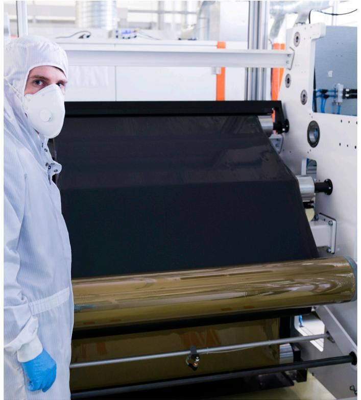
Flisom produces its solar modules using a roll-to-roll process. This means that at each process step, the one-meter-wide substrate web made of polymer is unrolled, processed and then rolled up again. Photo: Flisom
