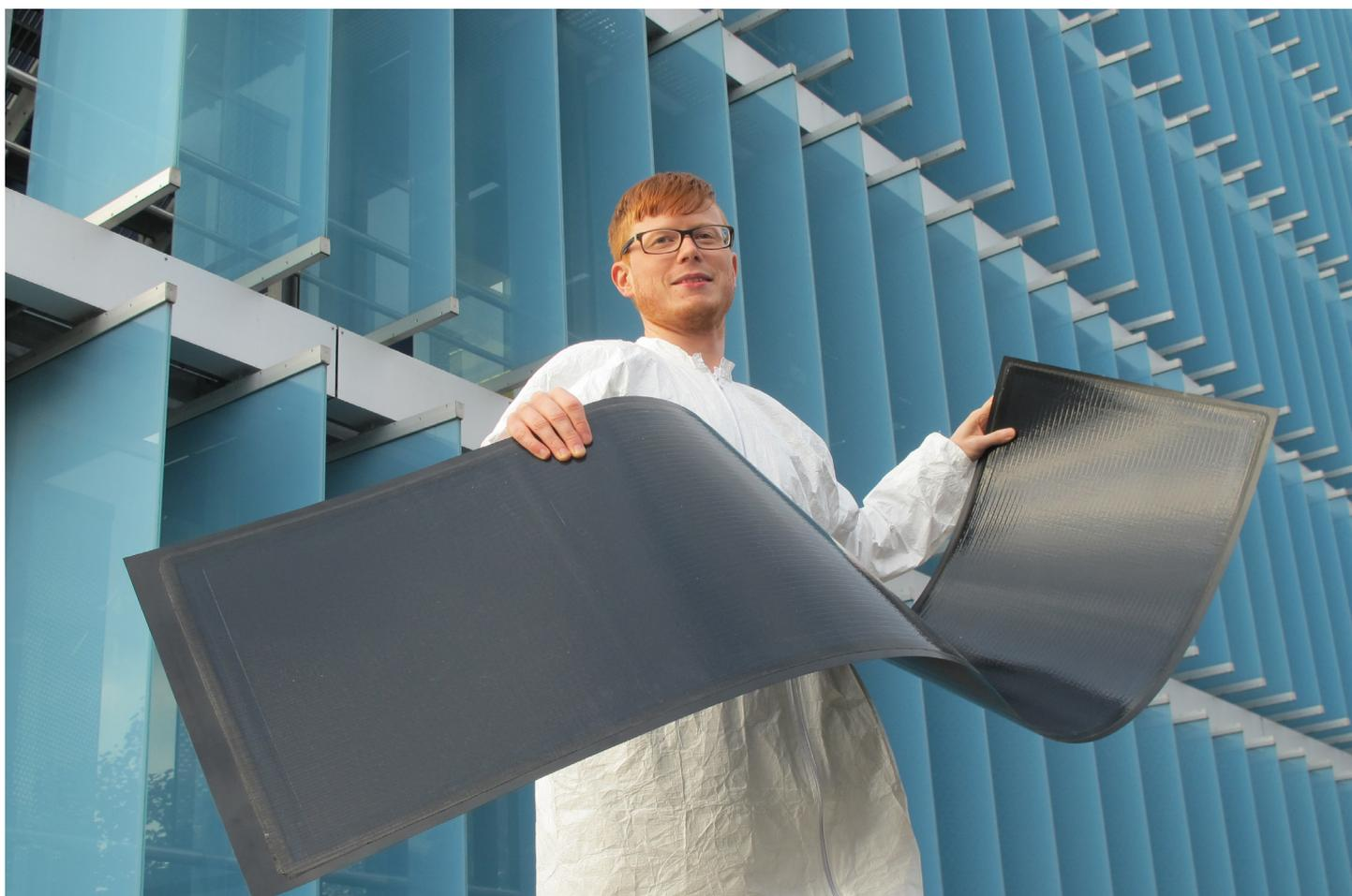
CIGS modules consist of a plastic film (polymer) that in several process steps is coated with photoactive materials. Photo: Flisom
