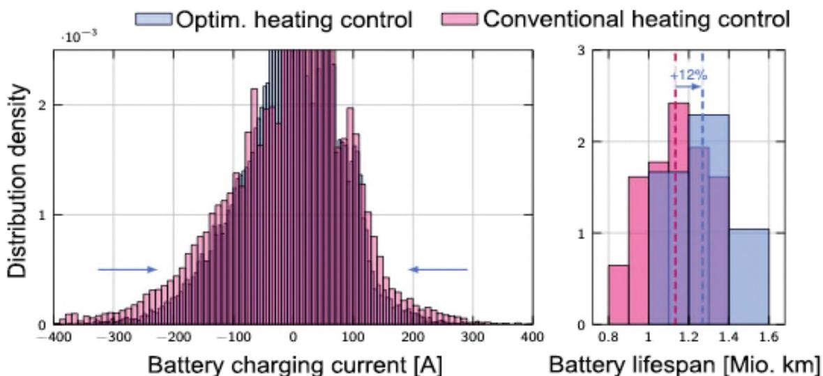
The graphic on the left shows that the heating control system developed at ETH can reduce high charge and discharge currents. This benefits battery life (graph on the right). Graphic: ISOTHERM final report
