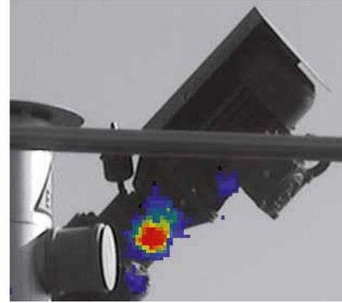
**Gas losses at the agitator of a biogas plant. The areas in red represent high methane concentrations, while areas in blue indicate low concentrations. Left: before lubrication; right: after lubrication.**
