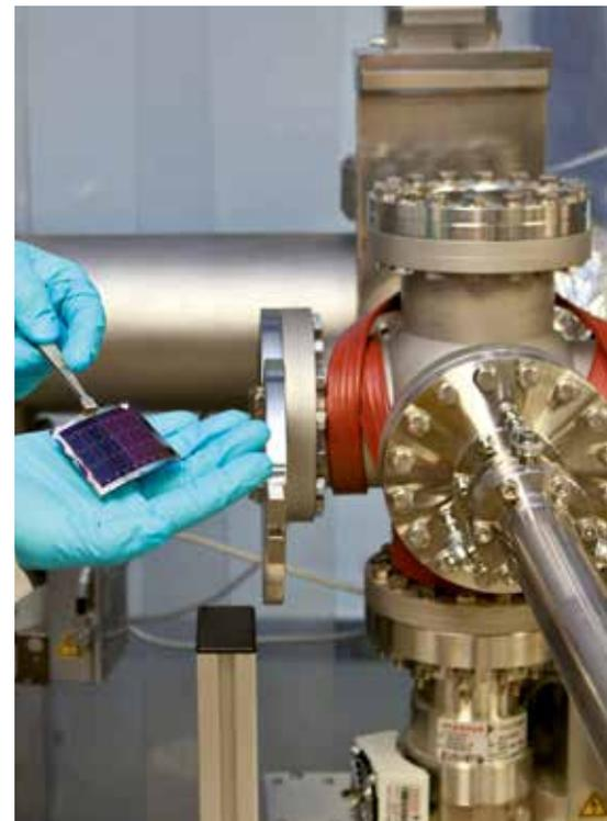
**Empa (Swiss Federal Laboratories for Materials Science and Technology) is one of the world's leading laboratories researching efficient CIGS thin-film solar cells. Since 1999, the degree of efficiency has been increased from around 13 percent to more than 20 percent in a series of development stages, with each stage representing a new record level worldwide.**
