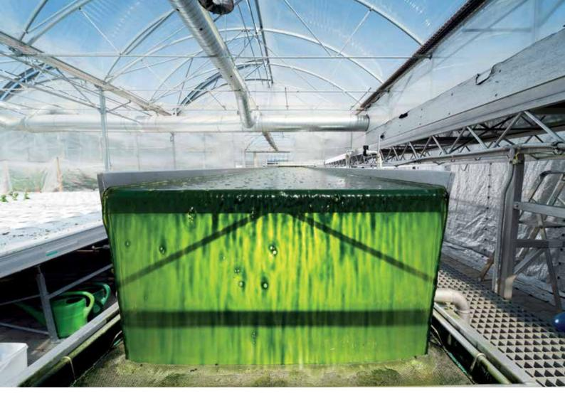
Production of "Chlorella vulgaris" blue-green algae in an open thin-film photo-bioreactor at the Zurich University of Applied Sciences (ZHAW).
