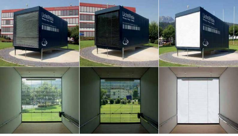
Container for measuring daylight illuminance set up at the Lucerne University of Applied Sciences and Arts in Horw: view of exterior (above) and interior (below).
