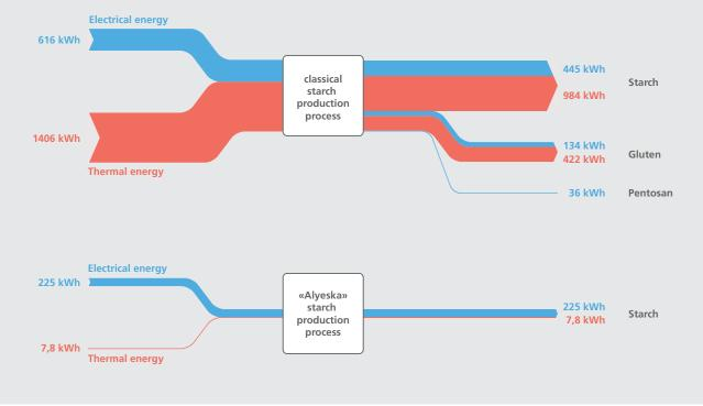
Sankey diagram relating to one tonne of starch product: the innovative "Alyeska" process for starch production requires significantly less heat (red) and electricity (blue) than the conventional starch production process.
