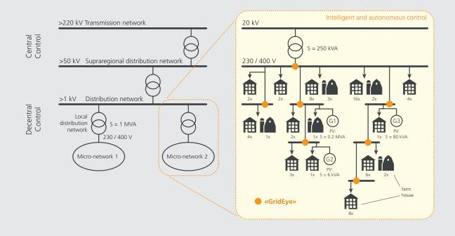
The "GridEye" system measures voltage at grid points in the distribution network and enables the optimum operation of the grid via a smart and autonomous control system.
