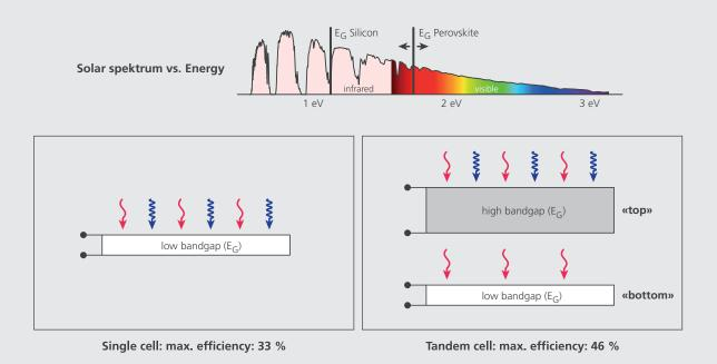
Single cells with one absorber (left) can only use the portion of the solar spectrum with energy larger than the band gap of the specific semiconductor material. Light with a "too high" energy level is transformed into heat. In a tandem cell (right), materials with differing band gaps are stacked so that the top cell absorbs in the blue range. The red light is transmitted and absorbed by the bottom cell.
