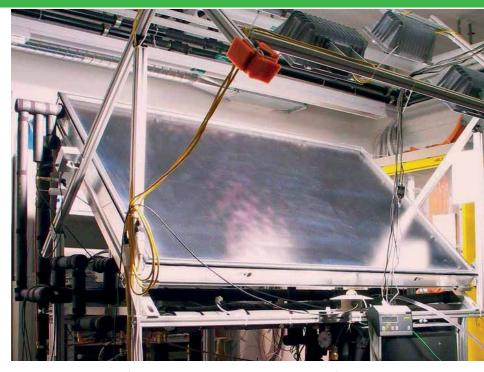
At the Federal Institute of Technology, Zurich, a new low-cost method for the solar thermal degasification of hydraulic circuits was developed and patented. Its feasibility was demonstrated on a test bench set up specifically for this purpose.
