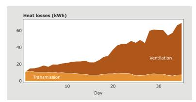
Only about 25 % of heat loss occurs through transmission (heat dissipation via the building envelope), the rest is at the expense of constant ventilation. More energy can be saved through heat recovery technology than through insulation of the building envelope.
