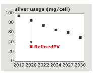
Silver consumption for silicon solar cells (monofacial, p-type) according to the International Technology Roadmap for Photovoltaic (ITRPV, 2020).
