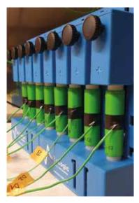
In a SFOE research project, test protocols have been developed that can provide the ageing status of battery cells in a few minutes, compared to the three to five hours required for a complete discharge/ charge cycle (source: CSEM).
