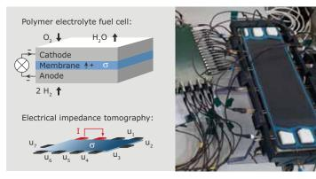
(Left) In order to examine the conductivity distribution  $\sigma$  in fuel cells by electrical impedance tomography, an alternating current I is applied between two electrodes (red) and the resulting changes in the surface potential are measured between pairs of electrodes. Repetition with many different configurations provides data from which the conductivity distribution in the membrane can be calculated. (Right) Experimental setup at the Paul Scherrer Institute.
