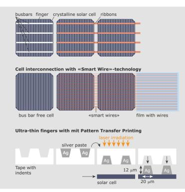
To contact crystalline silicon solar cells, metallic fingers and busbars are printed on the cells as current busbars. In recent years, technologies have been developed to connect cells without busbars and to reduce the width of the contact fingers. Both help to improve performance, as the cell is less shaded and there is less ohmic loss. Furthermore, silver is massively saved, which is a relevant cost factor.
