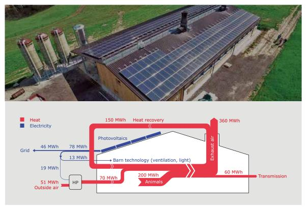
(Top) The Leuenberger fattening poultry house, Hellsau BE, 2019. (Bottom) Energy flow diagram for heat and electricity in a Minergie poultry farm (Data Hellsau).
