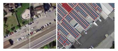
A decisive prerequisite for the identification of solar installations on aerial photographs is a correspondingly high resolution. The Federal Office of Topography swisstopo now provides images with a resolution of 10 cm. The left image illustrates this in comparison to the previous resolution of 25 cm (left part of the image). In order to train the neural network, a total of 7,839 images were prepared where photovoltaic and thermal plants were marked with polygons (source: FHNW).
