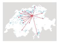
The basic idea behind solar forecasts based on "Big Data" is to make events in past PV production (e.g. clouds) informative for predicting production at other locations. The figure shows an example of a set of PV production locations for the prediction of a plant in central Switzerland.
