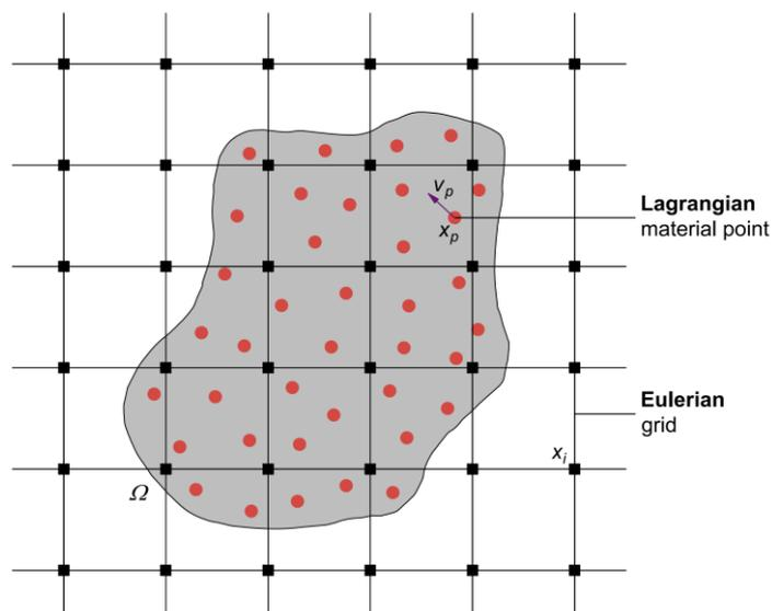
Figure 3.1: Lagrangian MPM discretization of a continuum and the Eulerian computational grid.
