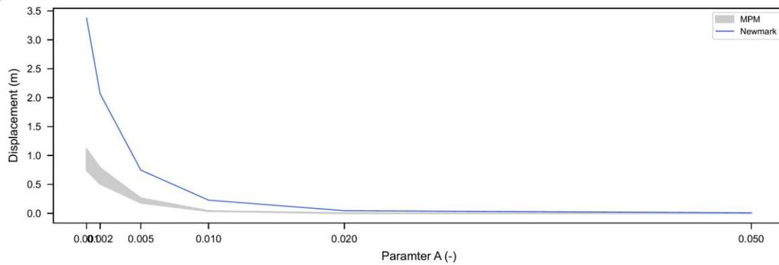
**Figure 5.6:** Co-seismic displacement for the Brienz landslide in Switzerland. (a) Geometry of the Brienz landslide. (b) and (c) comparison of the MPM simulation with a simplified Newmark for different rate dependency parameters A. The MPM simulation provides co-seismic displacements at each point of the landslide. The range of displacement is therefore represented as a hatch.
