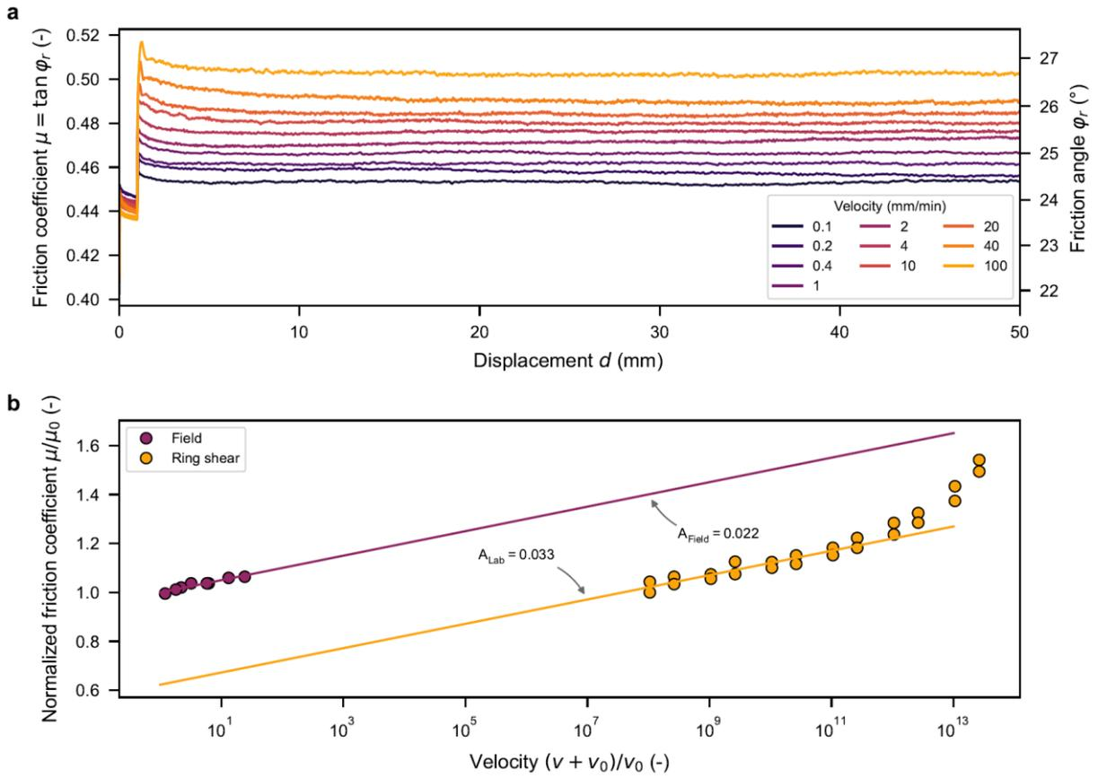
**Figure 3.8:** Ring shear tests results on samples from the shear zone of the Marsc landslide at different shearing velocities (a). Comparison of the rate dependency derived from field observations and lab testing (b). The ring shear test results from the three highest velocities are not considered for the regression to not overestimate the rate dependency at lower velocities.
