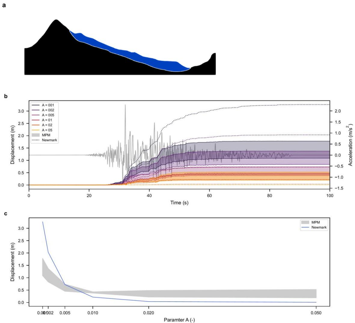
**Figure 5.5:** Co-seismic displacement for the Campo landslide in Switzerland. (a) Geometry of the Campo landslide. (b) and (c) comparison of the MPM simulation with a simplified Newmark for different rate dependency parameters A. The MPM simulation provides co-seismic displacements at each point of the landslide. The range of displacement is therefore represented as a hatch.
