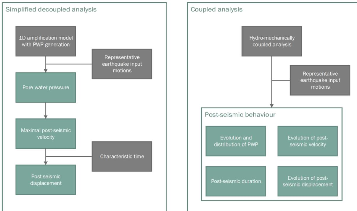
Figure 5.7: Procedure for the assessment of post-seismic displacements
