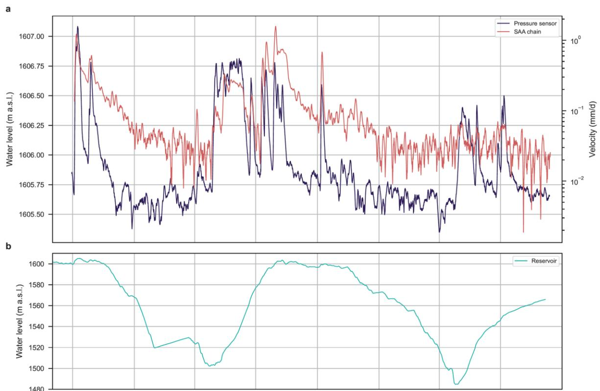
**Figure 3.4:** Measurements from Marsc landslide at the Luzzzone reservoir. (a) Water level in the landslide and the landslide velocity from SAA chain and (b) reservoir level.
