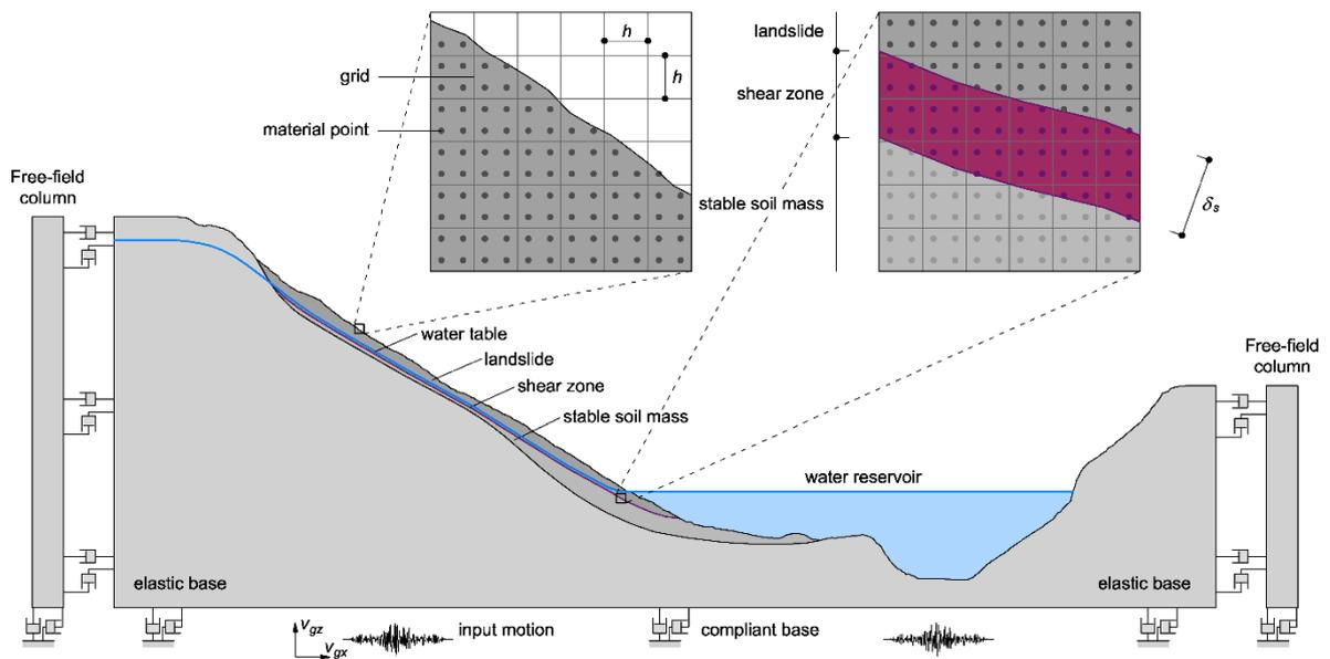
**Figure 3.3:** MPM landslide model. Schematic view of the MPM model of the landslide based on the Marsc landslide at the Luzzone reservoir, including the free-field columns at the lateral boundaries. The grid size is denoted with  $h$  and the thickness of the shear zone with  $\delta_s$ . The earthquake motion is applied by a vertical and horizontal component denoted with ground velocities  $v_{gz}$  and  $v_{gx}$ .
