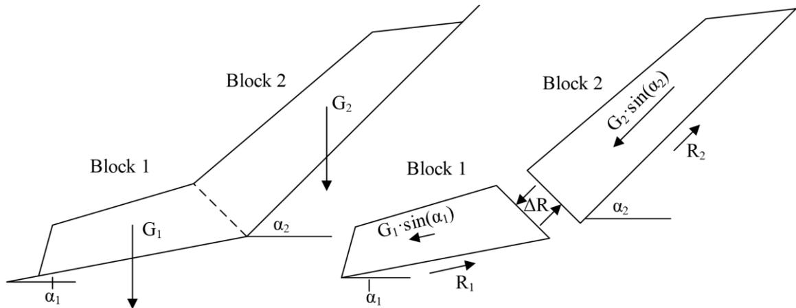
**Figure 2.2:** Simplified representation of landslide with varying inclination as two blocks.
