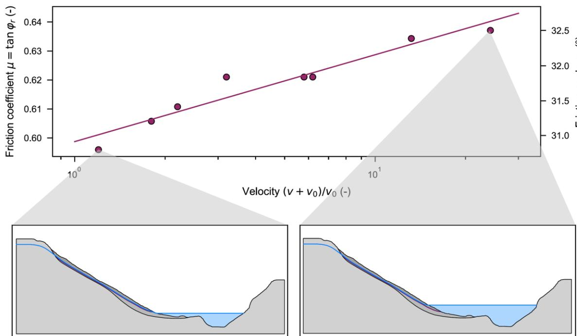
Figure 3.5: Calibration of the rate dependency in the shear zone using field measurements and the strength reduction method.
